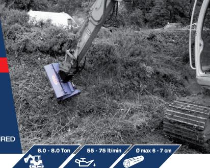
Flail mower head, for cutting grass, branches, bushes, dense vegetation, suitable to midiexcavators from 6,0 to 8,0 tons an power up to 70 hp. Max. cutting diameter 6-7 cm.
