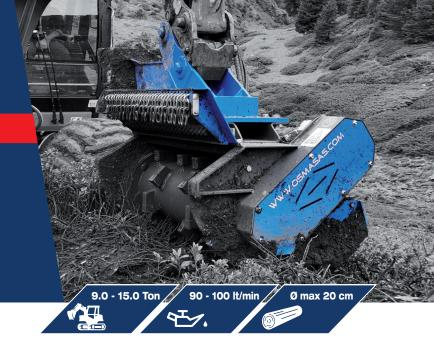
Midi-forestry mulcher for cutting grass, buses, branches, dense vegetation and small trees. Suitable on mini-excavator from 10,0 to 15,0 tons, with maximum power of 120hp, Max. cutting diameter 20cm.
