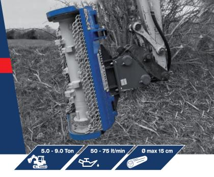
Midi-forestry mulcher for cutting grass, buses, branches, dense vegetation and small trees. Suitable on mini-excavator from 5,0 to 9,0 tons, with maximum power of 80hp, It can also fitted on boom mowers with piston pumps system. Max. cutting diameter 15cm.
