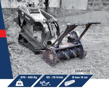
Forestry mulcher ideal for cutting shrubs, twigs and brambles, trees up to 15 cm high. DCR limiting rotor equipped with K-type fixed tools. It is applied to skid steer and compact loaders, and is suitable for working on uncultivated land, undergrowth and green areas in general, which require high power work.
