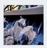
Rotor with steel profiles (DCR) for both types of tools
